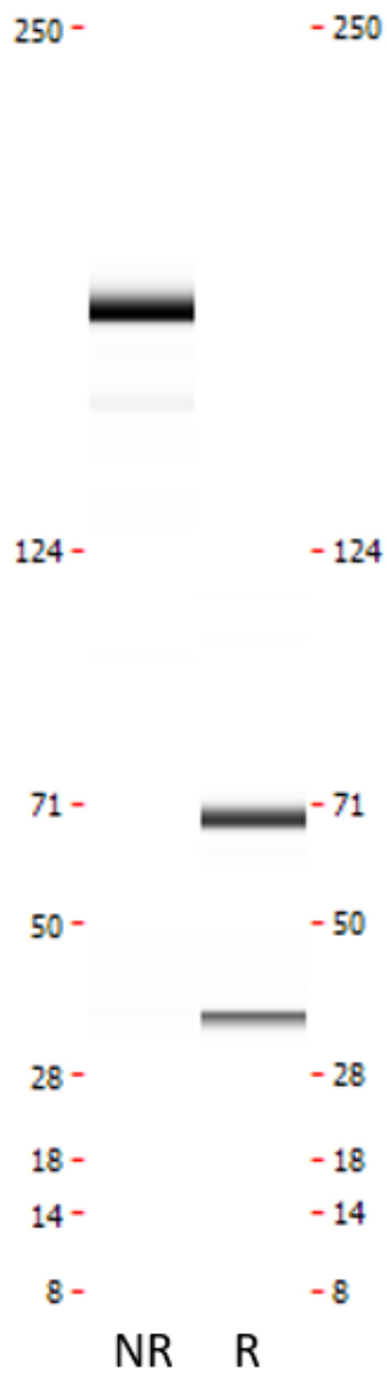
Figure 1. CE-SDS virtual gel output (LabChip GX) for monoclonal antibody to C-reactive protein, clone 9G8 under non-reduced (NR, left) and reduced (R, right) conditions.
