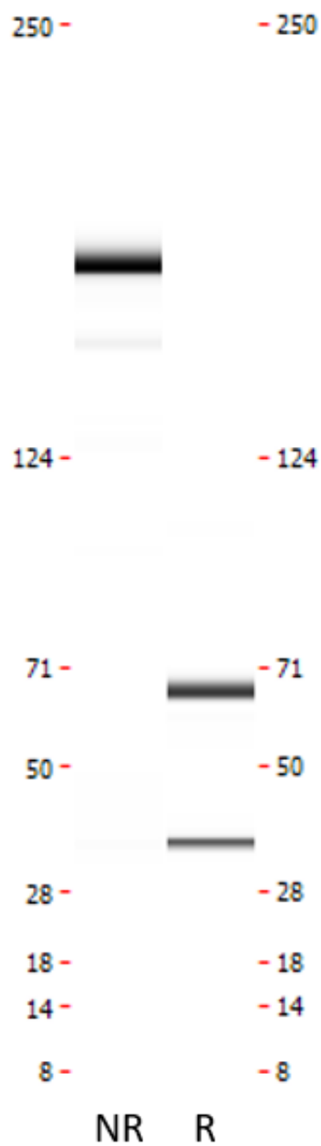
Figure 1. CE-SDS virtual gel output (LabChip GX) for monoclonal antibody to C-reactive protein, clone 6F6 under non-reduced (NR, left) and reduced (R, right) conditions.
