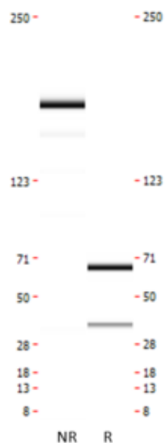
Figure 1. CE-SDS virtual gel output (LabChip GX) for monoclonal antibody to CHI3L1, clone 4G3 under non-reduced (NR, left) and reduced (R, right) conditions.
