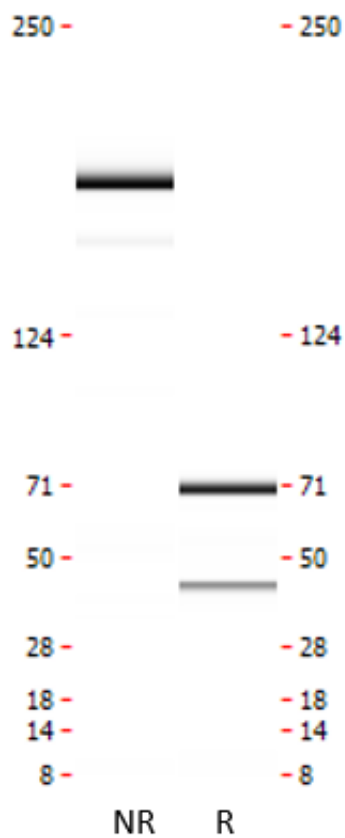
Figure 1. CE-SDS virtual gel output (LabChip GX) for monoclonal antibody to FGF-21, clone 9F5 under non-reduced (NR, left) and reduced (R, right) conditions.
