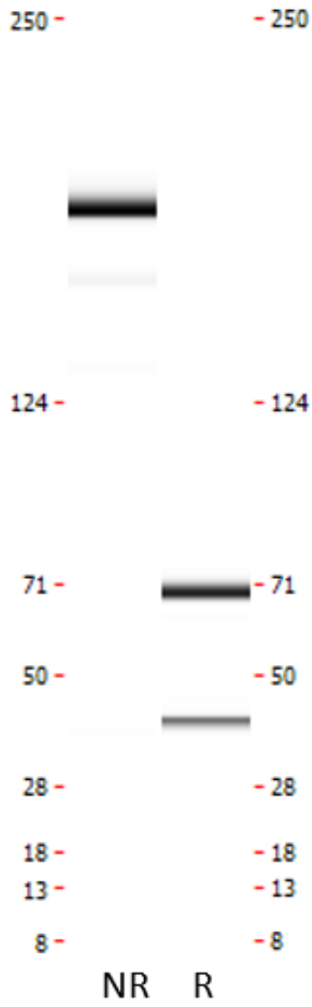
Figure 1. CE-SDS virtual gel output (LabChip GX) for monoclonal antibody to Cardiac troponin T, clone 3D3 under non-reduced (NR, left) and reduced (R, right) conditions.
